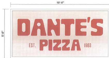
SIGN #1 Reface existing double face pole sign Optional: Non-illuminated or internally illuminated with LED Flat face with digital print graphics
